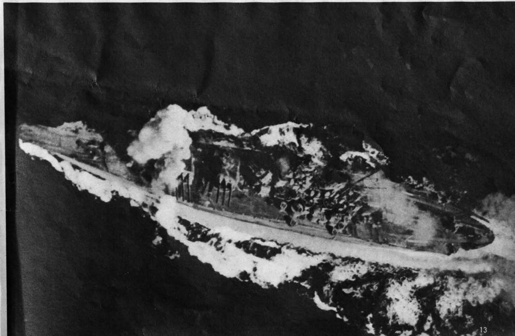
BOMBS BURST NEAR FORWARD TURRET OF YAMATO CLASS BB. NOTE SUPERFIRING TRIPLE SECONDARY, SINGLE STACK JUST FORWARD OF MAINMAST
